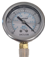
ILVG3025-4LNL GAUGE 2-1/2" Liquid Filled, 30-0, 1/4" MIPT Lower Connection
